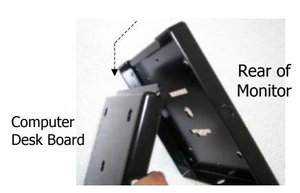
Once each of these parts are attached to the Computer Desk and to the Rear of the monitor, simply "hang" the monitor onto the computer desk mounted bracket and affix it into place by screwing the 3 black screws on the sides.
